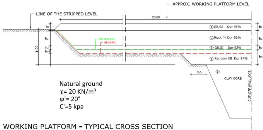
**Figure 7 Detailed design of working platform by BAUER**
