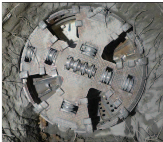
(e) Drill head of the TBM in the target cavern after it had drilled approximately 190 m through the tunnel.
