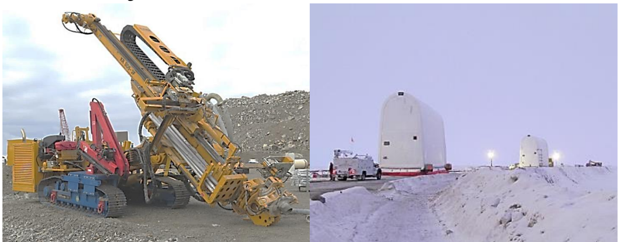
Figure 3. Klemm KR 806 drill rig on site and drill rig tents for winter period
