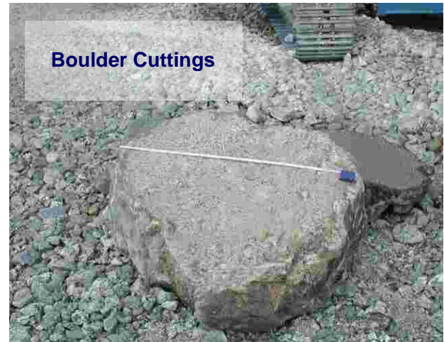
Figure 4. Cutting of cobbles and boulders
