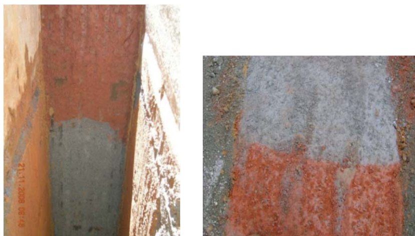
Figure 17. Dyed concrete for testing and confirmation of assumptions. Perfect quality of joints was proven.
