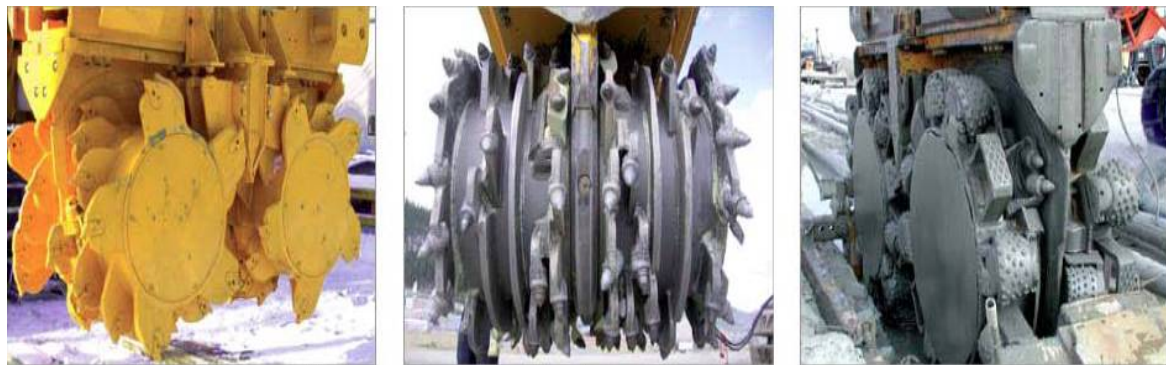
Figure 6. Wheel-sets (BAUER) for rock-cutting (soft-medium-hard)
