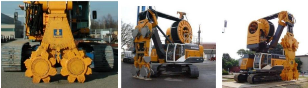
Figure 8: Cutter Soil Mixing equipment.
