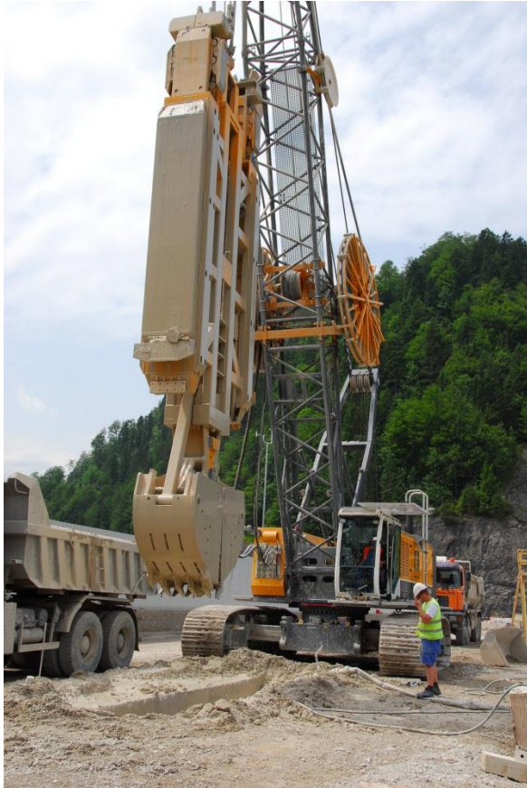
Fig. 5: The main equipment; left: BAUER MC 64 with hydraulic grab – right: BAUER MC 128 wit BC 40 Cutter
