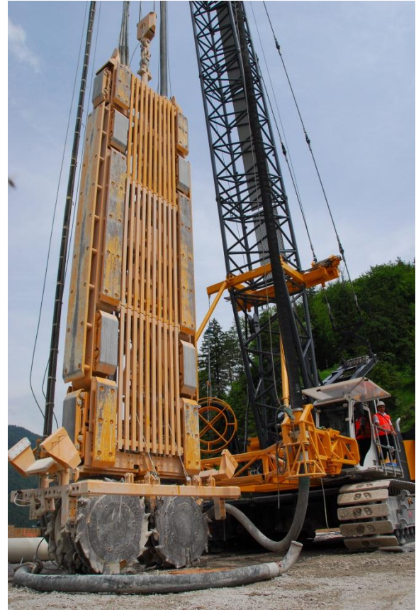
Fig. 5: The main equipment; left: BAUER MC 64 with hydraulic grab – right: BAUER MC 128 wit BC 40 Cutter
